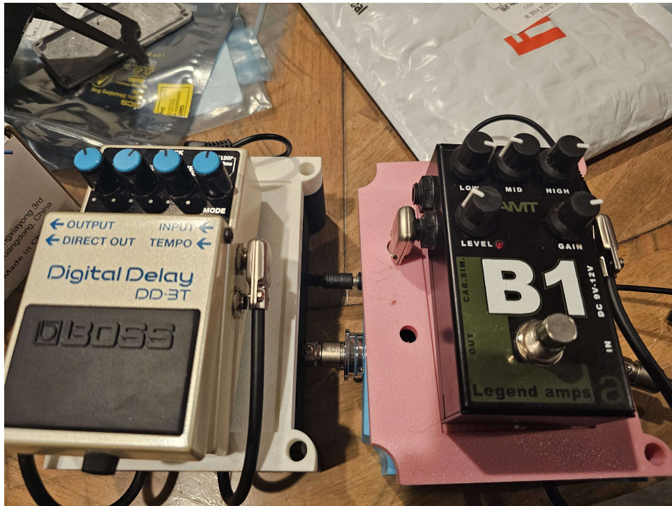
Figure 15: The Complete Central Controller with Two Mounted Pedals.
